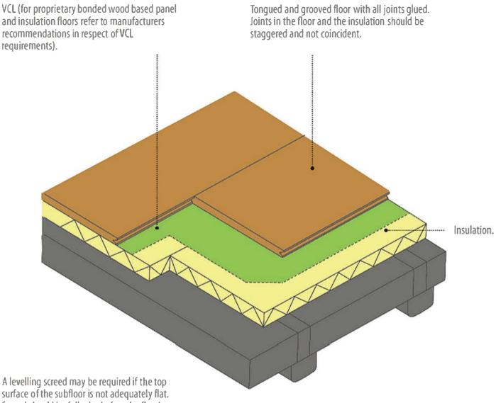
Screed should be fully dry before the floating floor is laid.
