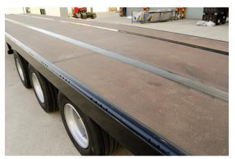
Figure 3.3: Flatbed truck using WISA bonded floor solution Photo: UPM-Kymmene Wood Oy
