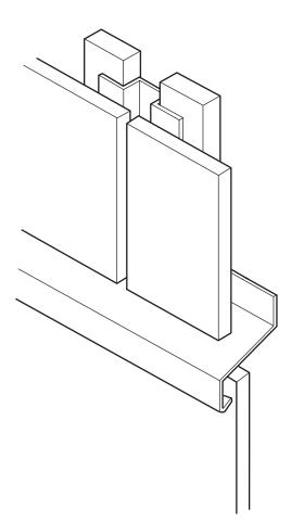
Figure 4.14: Vertical and horizontal external cladding joints using pressed metal 'top hat' and drained bottom bead profiles to allow drained and ventilated cladding
