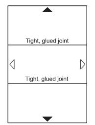
Figure 4.7b: Panels fixed as a composite unit with a movement gap at the perimeter
