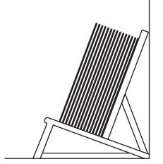
Figure 4.2: Correct method of edge stacking
