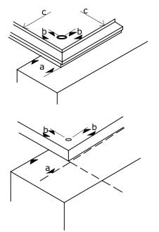
Figure 2.10: A minimum edge nailing distance of 8mm should be maintained and a minimum bearing of 18mm provided to each panel in both T&G panels (upper diagram) and square-edged panels (lower diagram)
