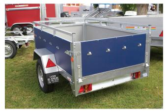
Figure 3.5: Car trailer using WISA Multiwall panels Photo: UPM-Kymmene Wood Oy
