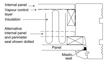
Figure 2.24: Infill panel with exposed framing
