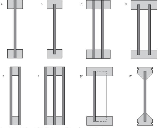
Figure 2.16: Typical forms of timber box beams and I-beams (\*patented designs)
