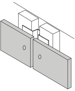
Figure 2.22: Open vertical joint with preformed metal 'top hat' flashing
