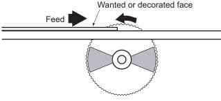
Figure 4.3: Sawing wood-based panels
