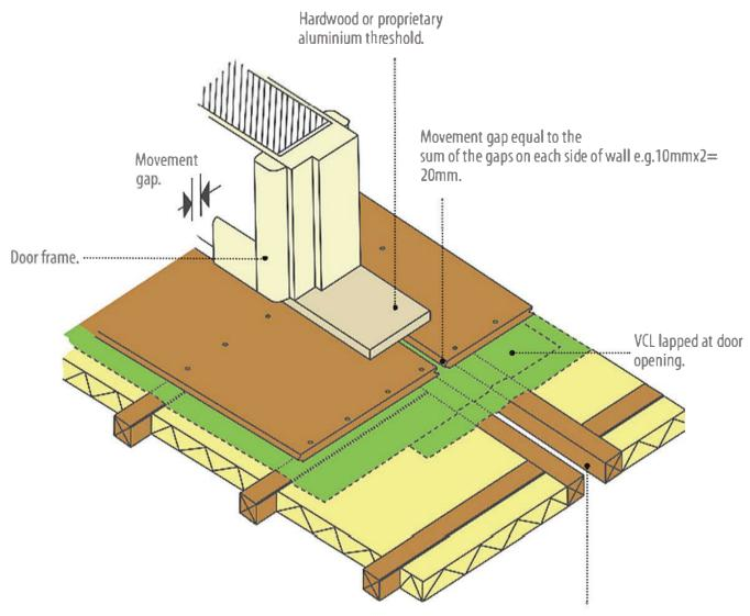
Battens for full width of door opening — gap between battens at least equal to gap between flooring boards.
