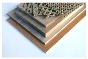
Figure 1.7: Dry process fibreboards
