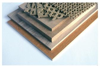
Figure A2.5: Dry process fibreboard (MDF)
