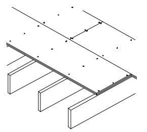
Figure 2.2: Tongued and grooved edge structural decking should be laid across the joists with short edges supported on joists
