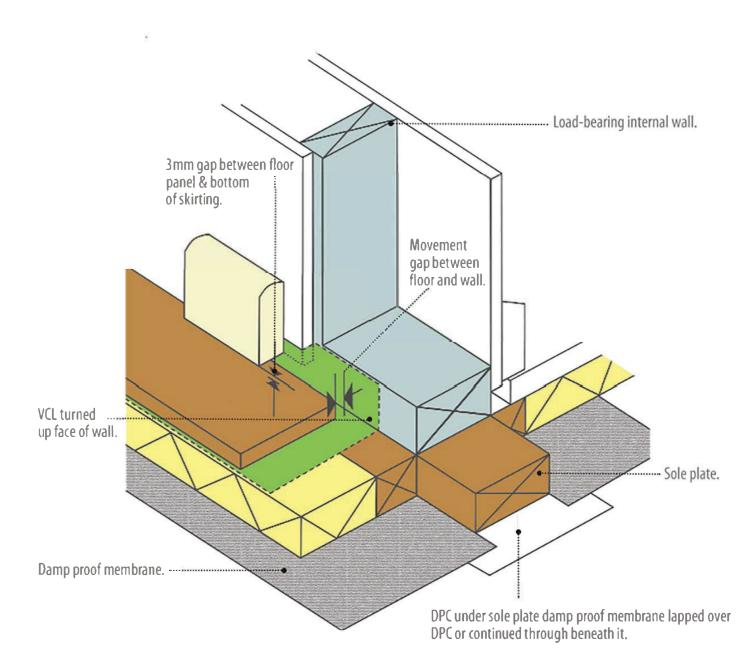
Figure 7: Detail at a load-bearing wall.
