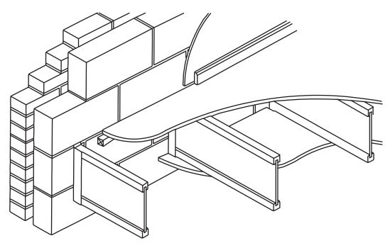
Figure 2.17: I-joists in block wall construction
