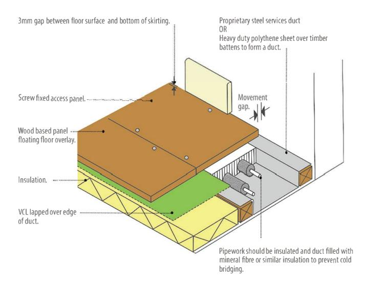
Figure 5: Typical service duct detail
