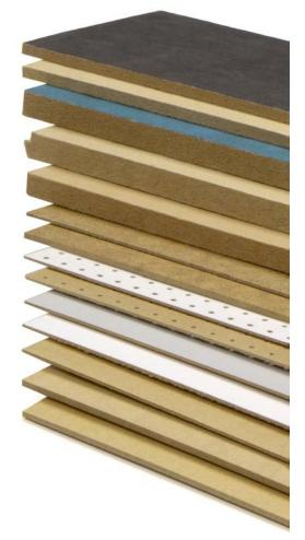
Figure 1.6: Wet process fibreboards
