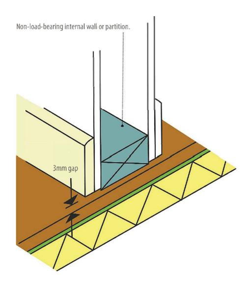
Floating floor continuous beneath wall.
