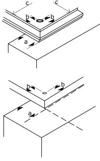
Figure 2.5: A minimum edge nailing distance of 8mm should be maintained and a minimum bearing of 18mm provided to each panel in both T&G panels (top) and square-edged panels (bottom)
