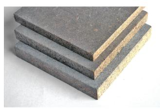
Figure A2.3: Cement-bonded particleboard
