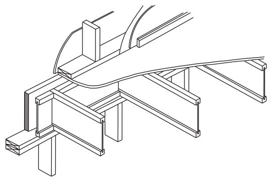
Figure 2.18: I-joists in timber frame construction
