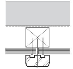
Figure 4.13: External cladding joint sealed with non-setting sealant, backed by foam breaker strip, and with timber cover strip to the joint
