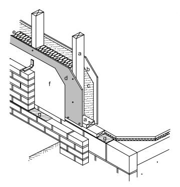
Figure 2.14: Typical timber frame external wall construction
