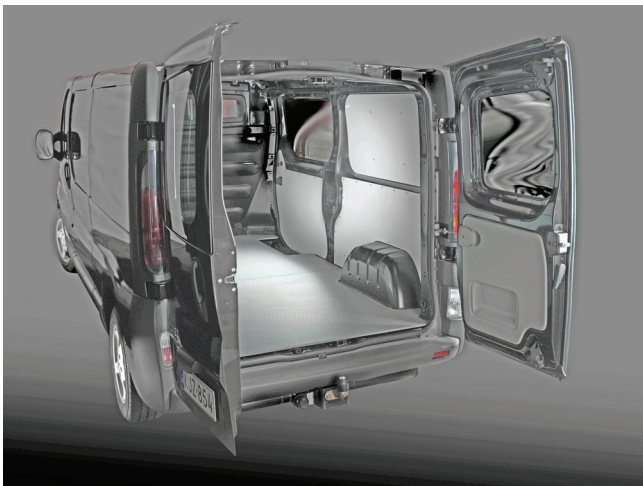
Figure 3.1: Van interior using WISA-Multifloor and WISA-Multiwall panel products Photo: UPM-Kymmene Wood Oy
