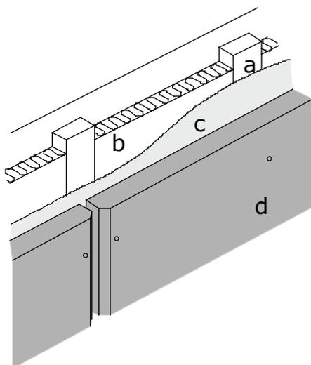
**Figure 2.29: Internal lining with thermal insulation**
