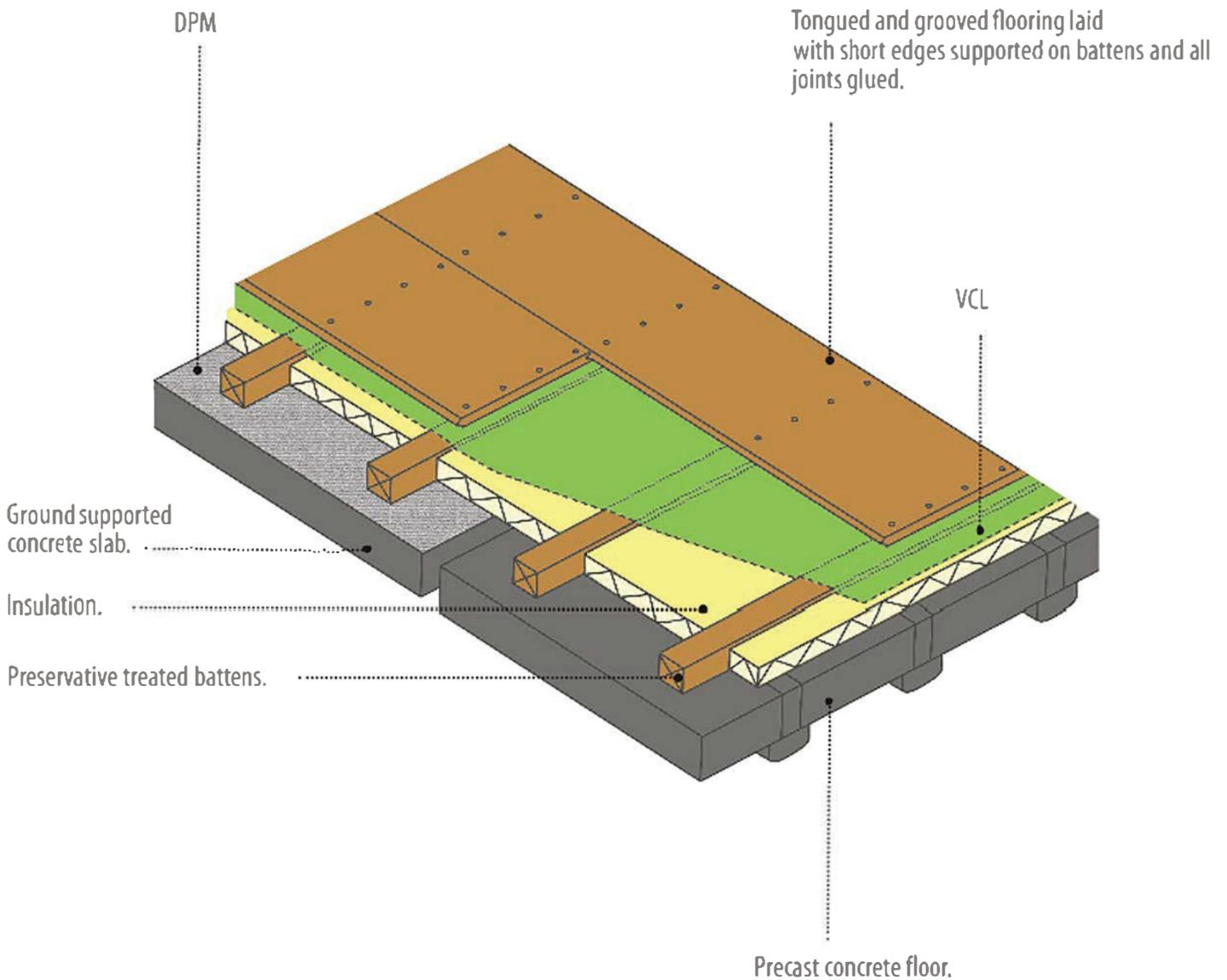
**Figure 9: Self-supporting OSB or particleboard floating floor over ground supported concrete slab and precast concrete floor.**
