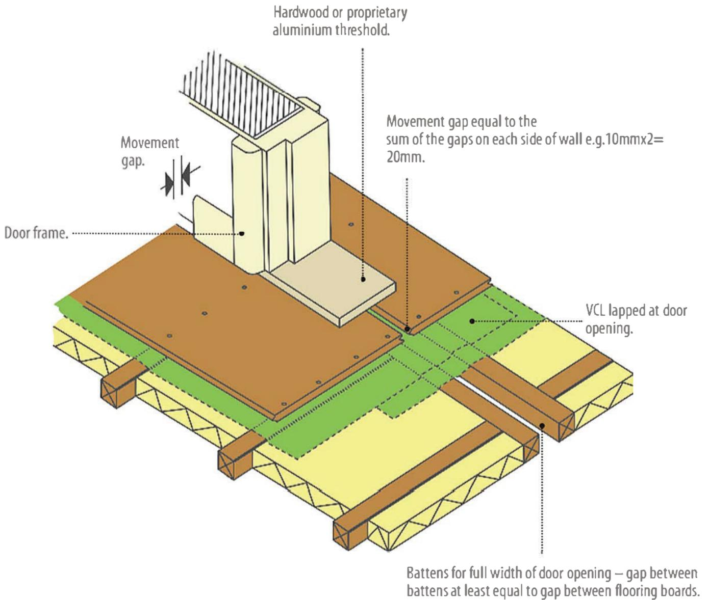
**Figure 11: Detail of the threshold of a doorway in a wall which is built off the supporting concrete structure when a battened floor is used.**
