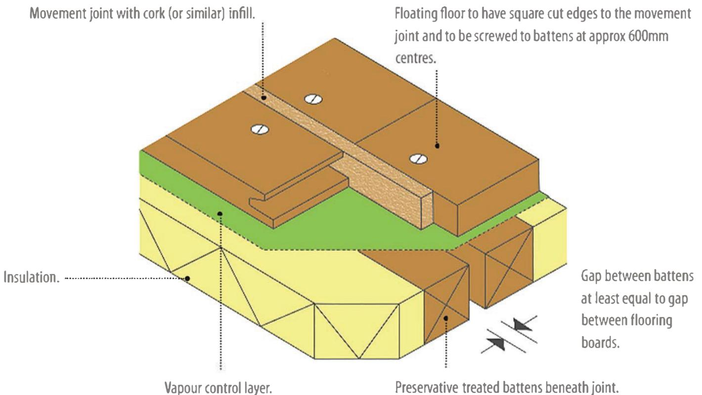
**Figure 4: Detail of typical intermediate movement joint**
