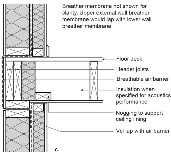
**Figure 2.4: Floor/external wall junction showing panel extending beyond room perimeter under the wall**
