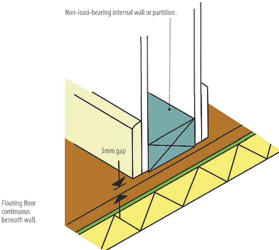
**Figure 8: Supporting a non-load-bearing wall.**
