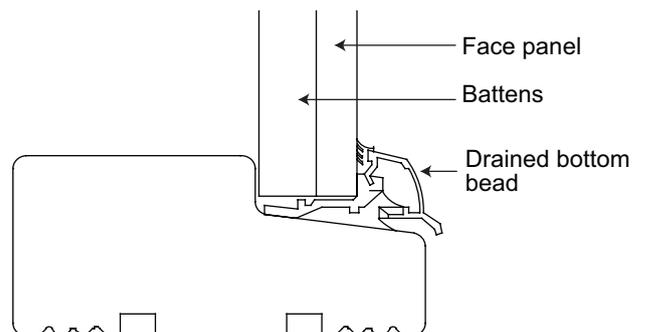
**Figure 2.24: Infill panel with exposed framing**
