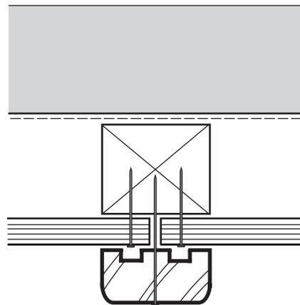
**Figure 2.21: Board cladding with vertical battened joints**
