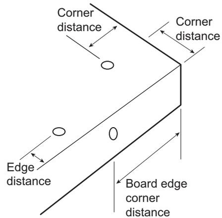
Figure 4.12: Fixing positions
