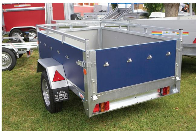
**Figure 3.5: Car trailer using WISA Multiwall panels**
