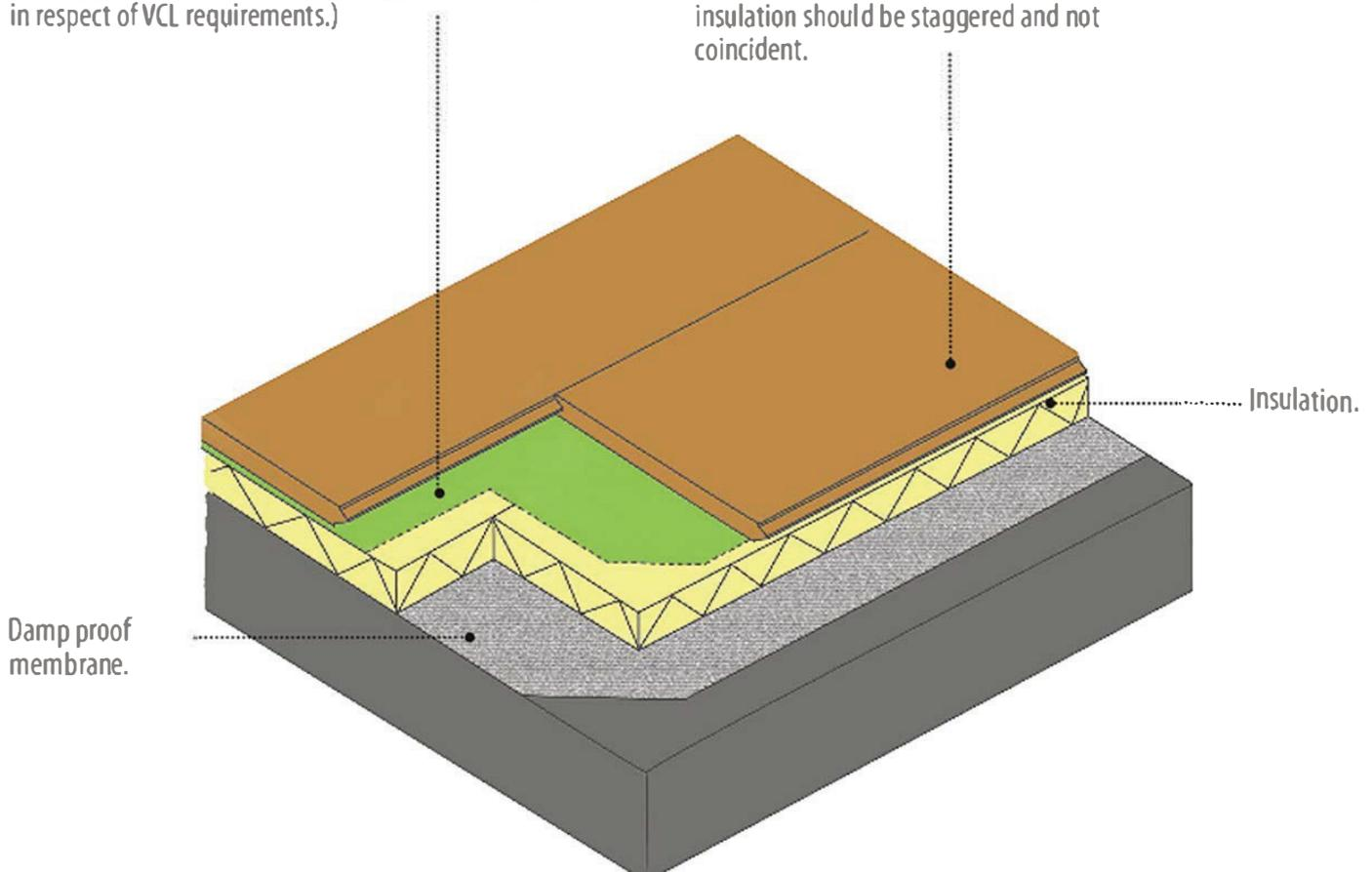
**Figure 1: Floating floor on an in situ concrete slab**
