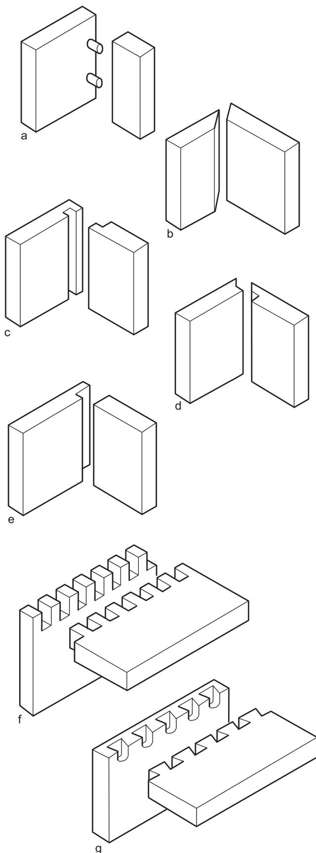
**Figure 4.16: Typical joints used in furniture construction**
