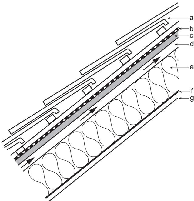
**Figure 2.12: Example of a warm roof with sloping ceiling and insulation between rafters. There must be adequate ventilation above the insulation**
