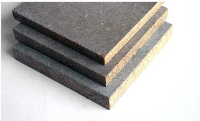
Figure 1.5: Cement-bonded particleboard
