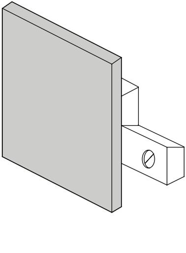
**Figure 2.27: Secret fixing using interlocking battens**
