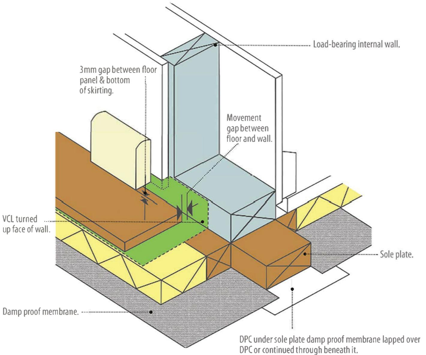
**Figure 7: Detail at a load-bearing wall.**
