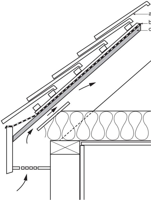
**Figure 2.11: Example of a cold roof space with insulation at ceiling level. The roof space must be adequately ventilated**
