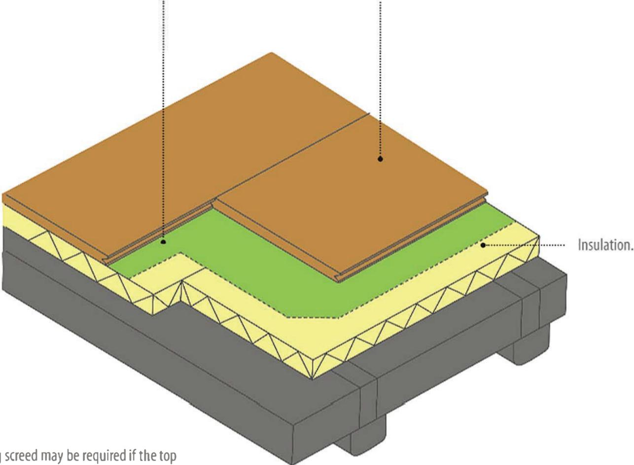
A levelling screed may be required if the top surface of the subfloor is not adequately flat. Screed should be fully dry before the floating floor is laid.
