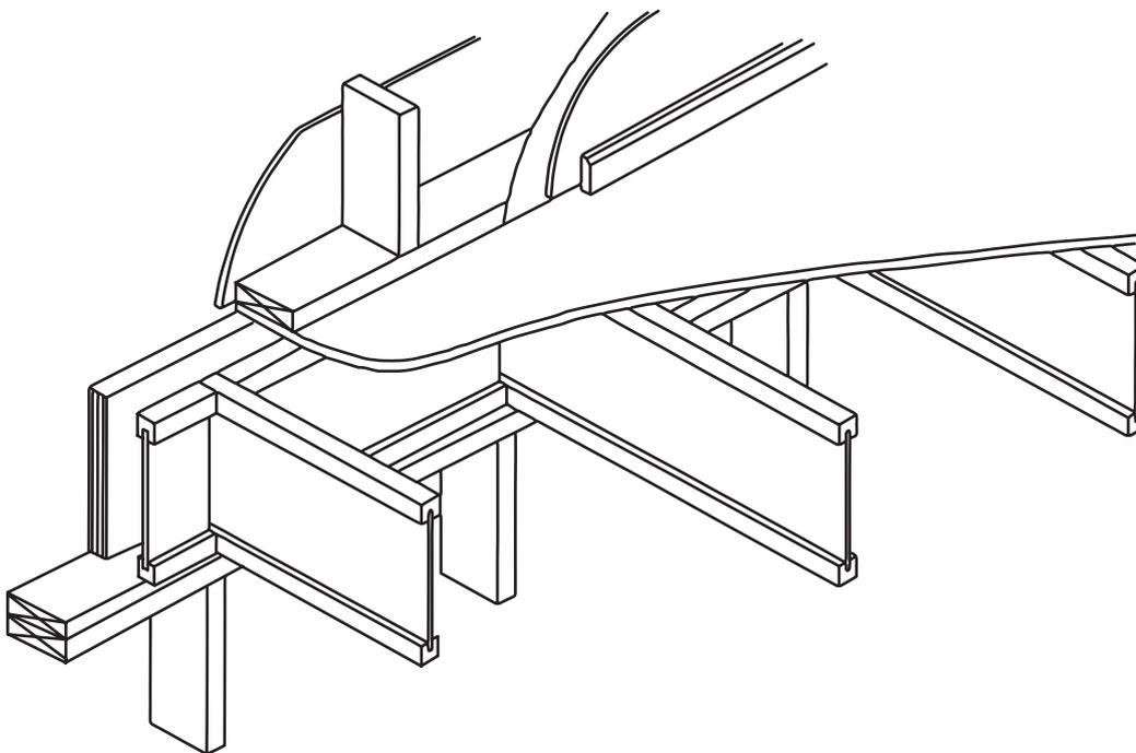
Figure 2.18: I-joists in timber frame construction
