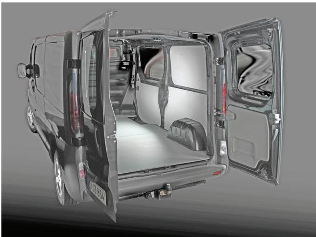
**Figure 3.1: Van interior using WISA-Multifloor and WISA-Multiwall panel products**
