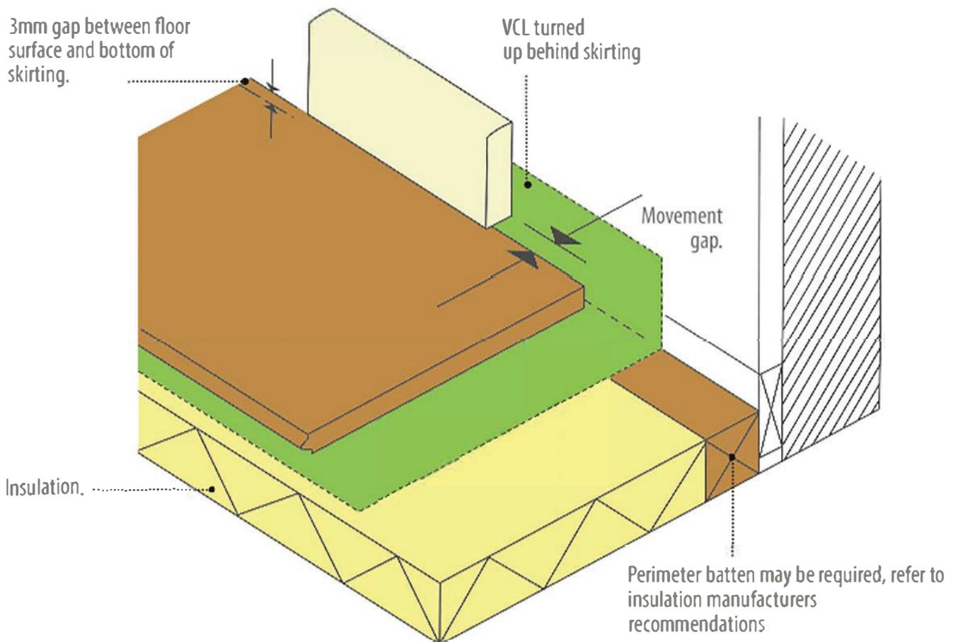
**Figure 3: Detail of perimeter floor**
