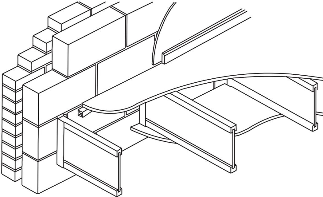
Figure 2.17: I-joists in block wall construction
