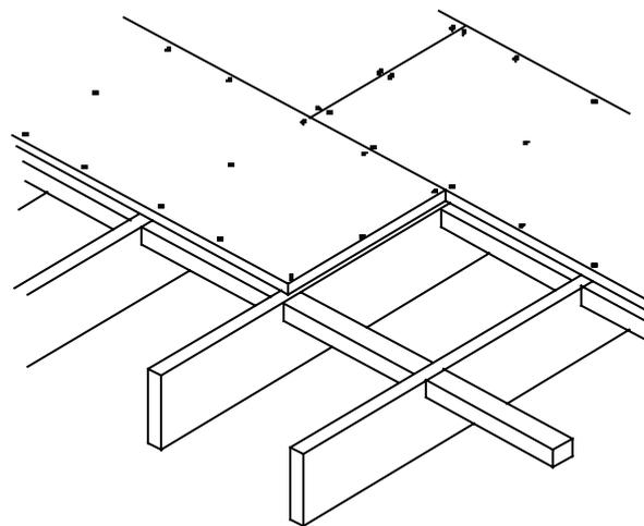
**Figure 2.3: Square edge structural decking laid across the joists and supported by noggings**
