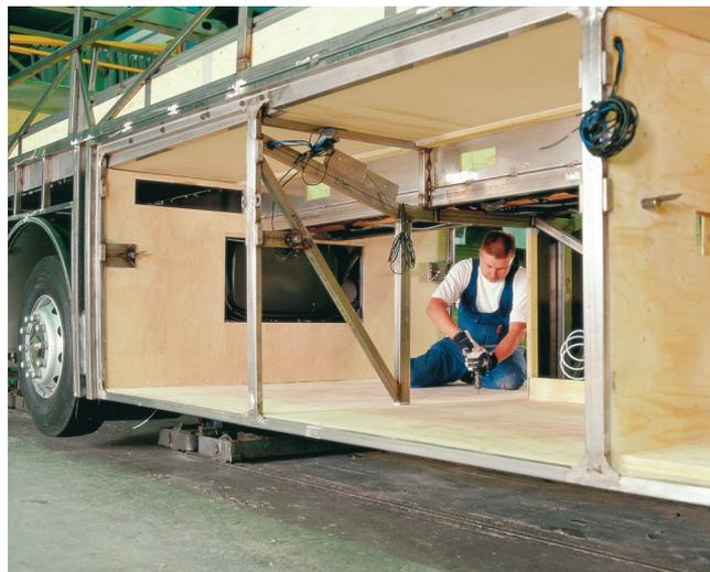
**Figure 3.6: WISA Birch panels installed in a bus**
