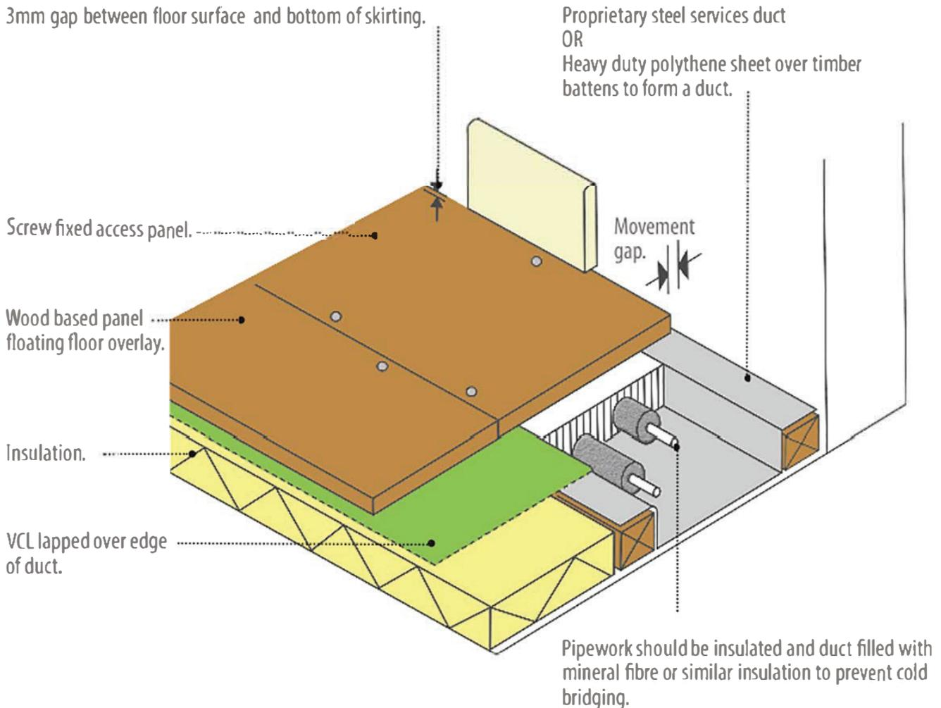
**Figure 5: Typical service duct detail**
