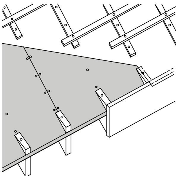
**Figure 2.13: Typical pitched roof with sarking board and tiling underlay beneath the counter battens**
