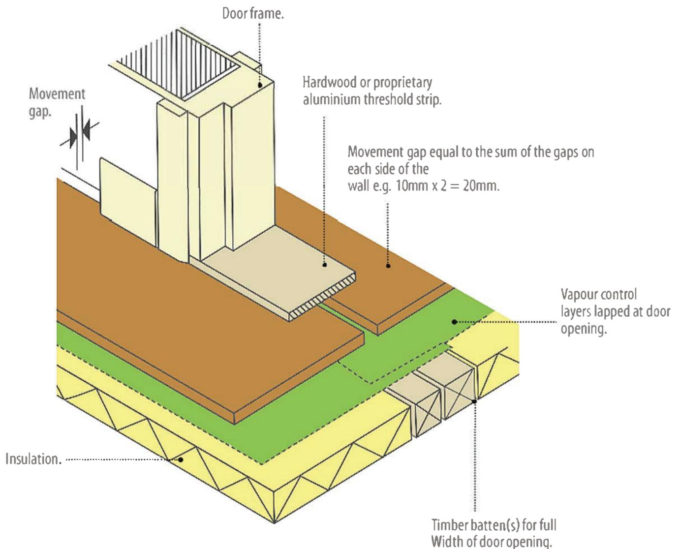
**Figure 6: Details at the threshold of a doorway in a wall which is built off the supporting concrete structure when a continuously supported floor is used.**
