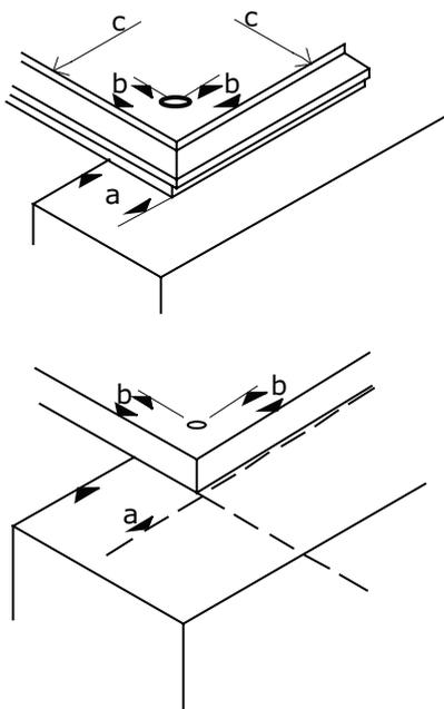
Figure 2.10: A minimum edge nailing distance of 8mm should be maintained and a minimum bearing of 18mm provided to each panel in both T&G panels (upper diagram) and square-edged panels (lower diagram)
