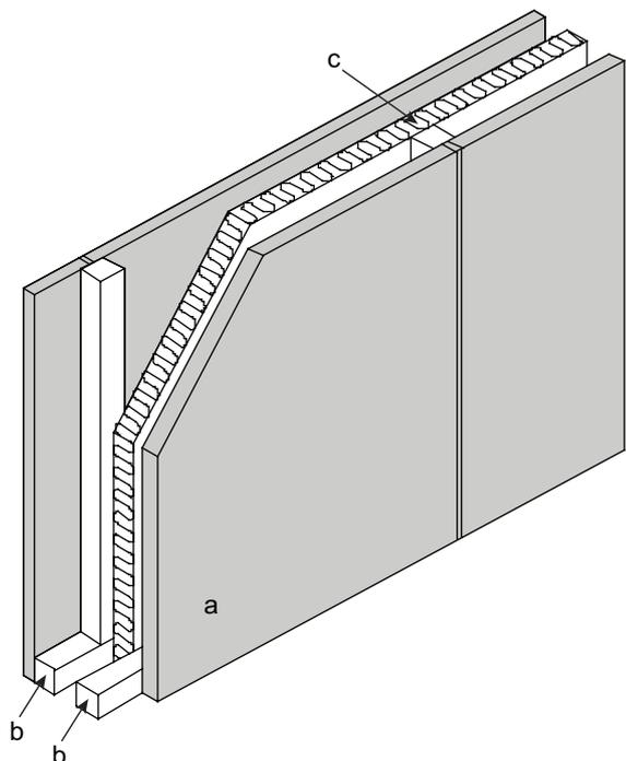
**Figure 2.26: Internal partition wall with improved acoustic performance**
