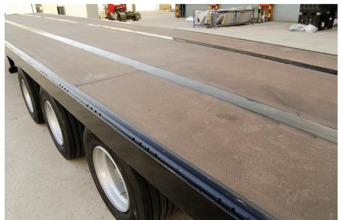
**Figure 3.3: Flatbed truck using WISA bonded floor solution**
