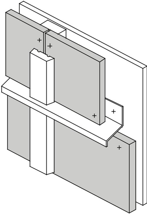
**Figure 2.23: Vertical joint with timber cover battens and horizontal joint with preformed metal flashing**
