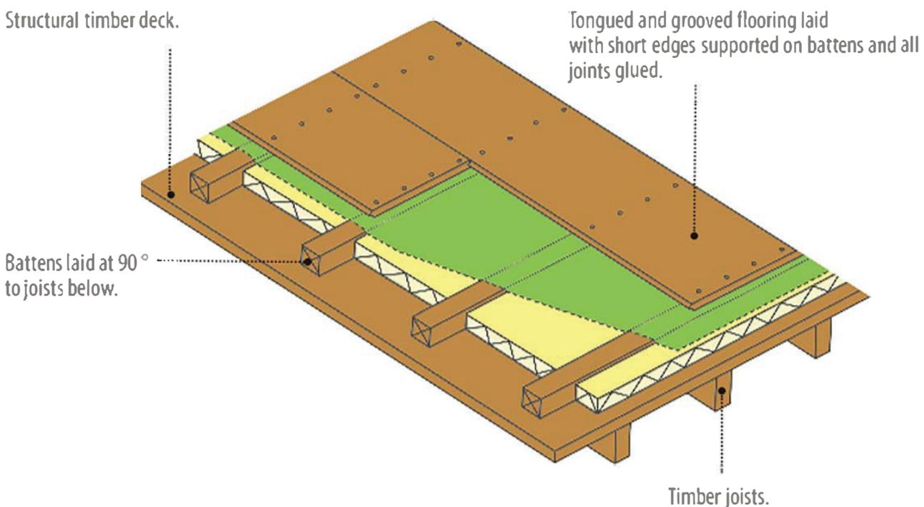
**Figure 10: Self-supporting OSB or particleboard floating floor over timber sub-floor.**
