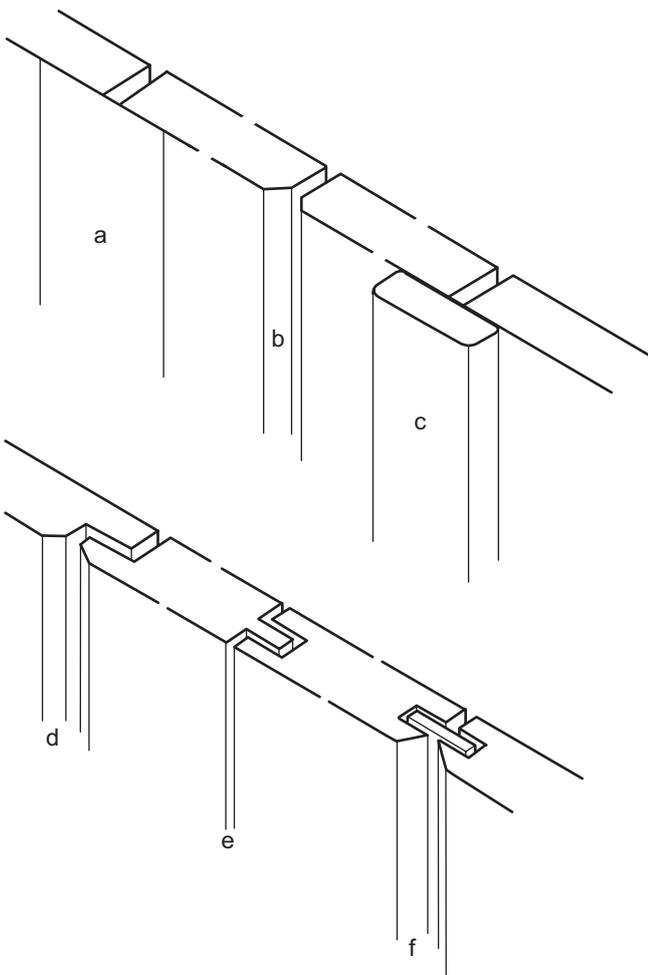
**Figure 2.28 :Typical lining panel joints**
